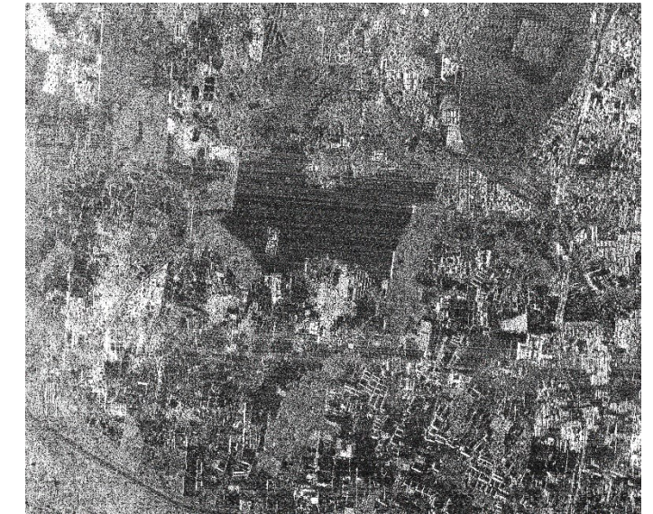
Interference in ISRO's P band airborne SAR, Hyderabad
