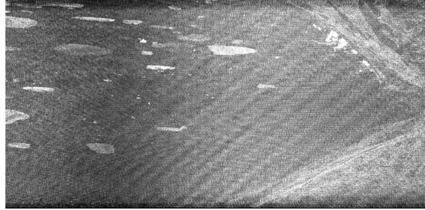
Interference in L band ALOS PALSAR data over Alaska Barrow
